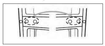
6. Unscrew bottom hinge. Then remove the adjustable feet from both sides.
