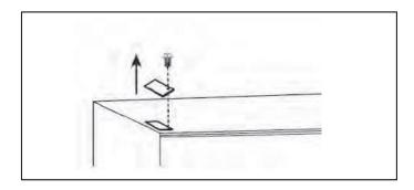
3. Unscrew the middle hinge. Lift the refrigerator door and place it in a safe place to protect it from damage and scratches.
