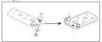
8. Transfer the lower door hinge to the proper position. Replace both adjustable feet.
