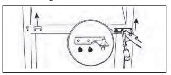
4. Move the shaft sleeve and the pinhole plug from left side to right side.
