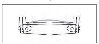
10. Reverse the direction of the middle hinge 180° and then move it to the left side of the refrigerator. Insert the middle hinge pin in the upper hole of the lower door and tighten the screws.
