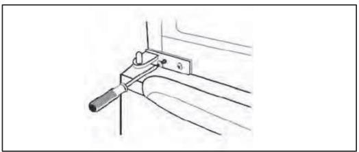
11. Place the upper door back on. Ensure the door is aligned horizontally and vertically so that it seals properly. Insert the middle hinge pin in the upper hole of the lower door and tighten the screws.
