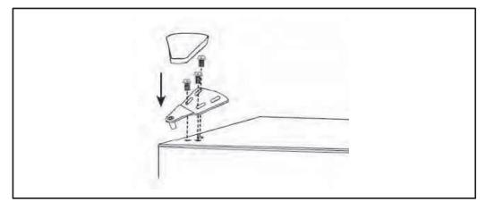
12. Move the hole cover from the left side to the right side and tighten it with a screw.
