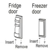
7. Place the freezer door on the middle hinge, making sure that the hinge pin is inserted in the hole at the bottom of the freezer door. Then replace upper hinge so it aligns with the door and screw into place. Replace hinge cover supplied with user manual and accessories.
