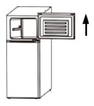
3. Using a screwdriver, remove the middle hinge. Lift the door upwards to disengage it from the lower hinge. Lay the door down gently on a padded surface. NOTE: The hole coverings on the bottom left of the refrigerator should be moved to the bottom right once the door is switched.
