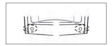
11. Place the upper door back on. Ensure the door is aligned horizontally and vertically so that it seals properly. Insert the middle hinge pin in the upper hole of the lower door and tighten the screws. 10. Reverse the direction of the middle hinge 180° and then move it to the left side of the refrigerator. Insert the middle hinge pin in the upper hole of the lower door and tighten the screws.
