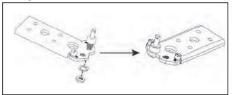
4. Move the shaft sleeve and the pinhole plug from left side to right side.
