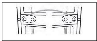
7. Remove the washer and nut that secure the hinge pin to the hinge, then move the pin and screws with the washer and nut into to left hole hinge.
