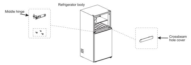
8) Place the freezer door on the middle hinge and install the top hinge; install the left top hinge cover on the right top side; install the top hinge cover on the left top side.
