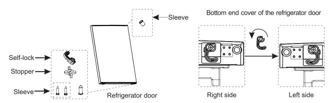
7) Install the replaced refrigerated door on the bottom hinge, then install the middle hinge and cover with the cross beam hole cover.
