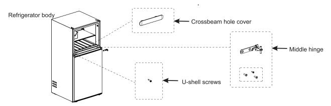
4) Take off the refrigerator door carefully (ensure not to lose small parts like sleeve and stopper on the door); Remove the bottom hinge and leveling foot. Remove the bottom hinge stop and the hinge shaft and install them on the other side of the hinge, and install the modified bottom hinge on the other side of the refrigerator; the leveling foot is installed on the original bottom hinge side.
