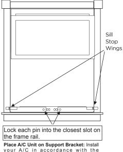
Place A/C Unit on Support Bracket: Install your A/C in accordance with the manufacturer's instructions and local and state ordinances. Be sure to provide a means to prevent the single or double hung sash from being opened above air conditioner.
